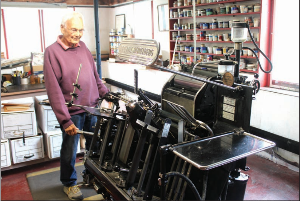
Darrell Hyder demonstrated the use of his original Heidelberg machine press in his workshop.
