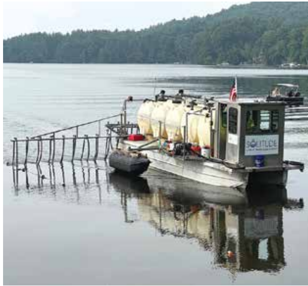
SOLitude's alum distribution barge pulls into the South Pond beach to refill. SUBMITTED PHOTOS
