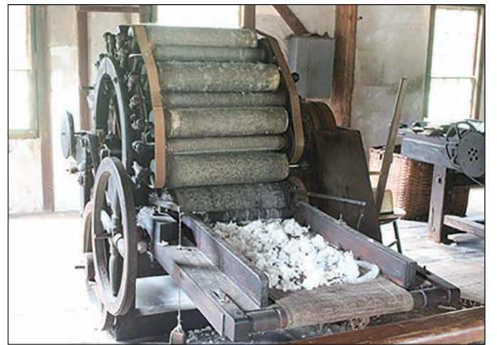
The carding machine from the early 1800s was running inside Old Sturbridge Village's Carding Mill.
